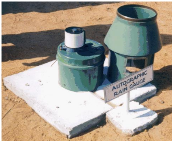
Fig. 1.2 A self recording rain gage with chart mounted on a drum (top) and rainfall recorded by the instrument on a chart.
